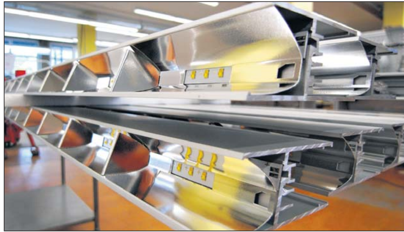
LED-Schienen in der Endmontage.
